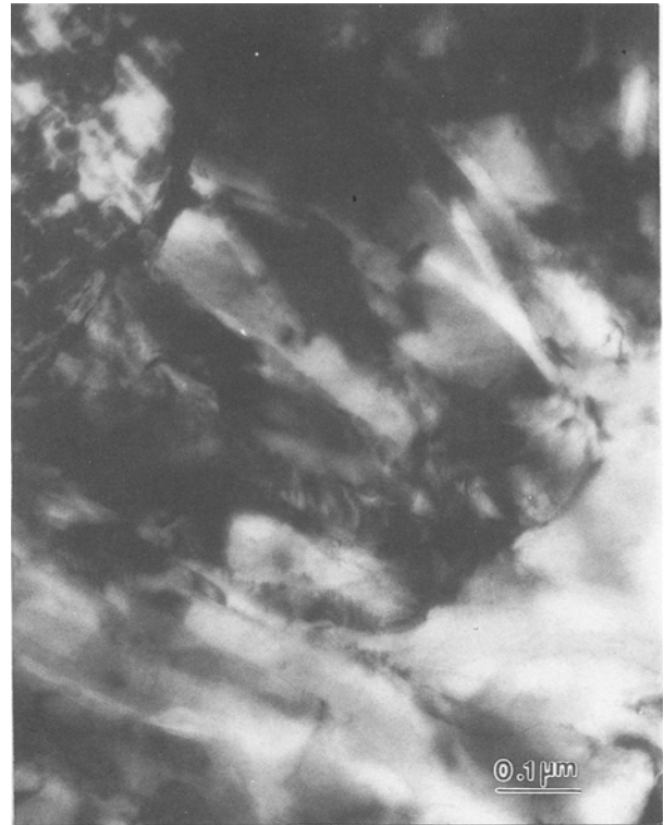
Figure 5 Bright-field image of the eutectic area.
